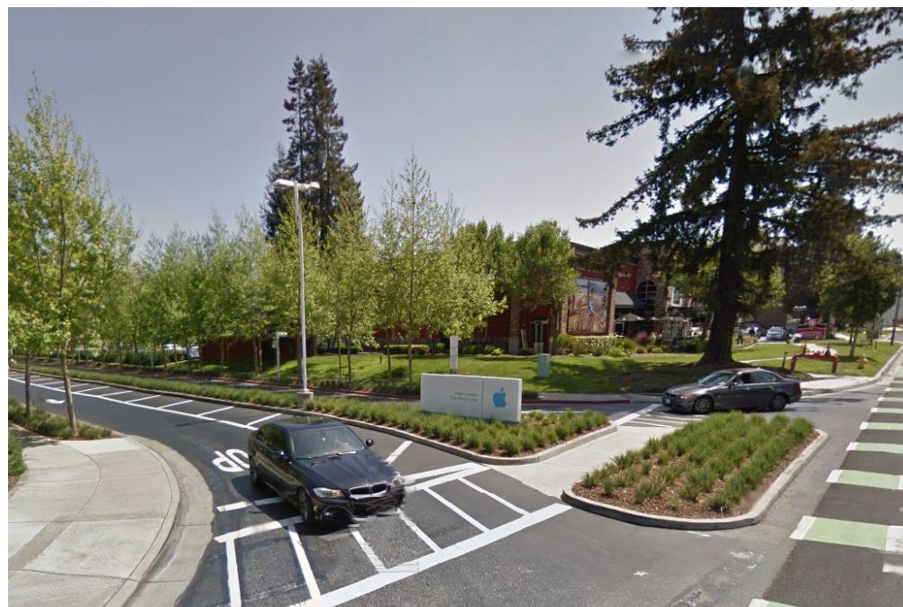
The sign should be oriented for greatest legibility from the street, and the scale of the entry drive should slow traffic.
