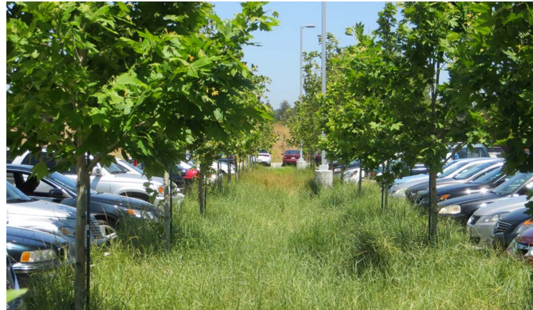
The permeable areas should be designed to hold and treat stormwater before it flows into the municipal system.
