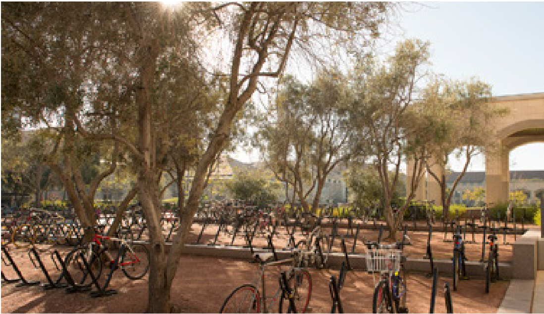
Decomposed granite and site walls delineate the bicycle parking area, and trees provide shade and a garden-like atmosphere.
